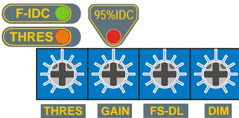
The system requires no trimming from the factory. If the user wants to alter the flow and other parameters, just use a small screw driver to complete the task. Below are the working details of each trimmer. (left to right).
