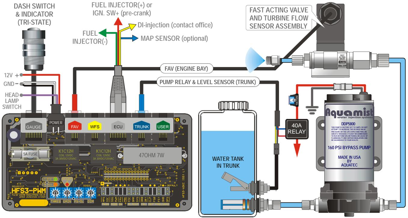
Note: Please ensure the correct harness is plugged into the appropriate socket to avoid causing permanent damage to the Electronic controller. The potentiometers on the controller are preset to mid-position from factory. System triggers at 40% of IDC. Fuel-IDC to Water-IDC ratio is 1. The system will operate correctly without any adjustments.
